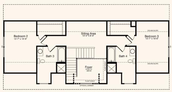
FOR SECOND FLOOR LIVING AREA ALL DESIGN, MATERIALS, AND WORK TO BE THE RESPONSIBILITY OF THE BUILDER ON SITE. INSULATION MUST REMAIN R-30 IN THE ROOF AND R-13 IN THE WALLS. LIGHT, VENT & EGRESS IS THE RESPONSIBILITY OF THE BUILDER ON SITE.
